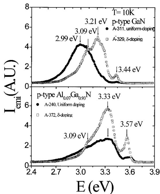
FIG. 4. Comparison of low-temperature (10 K) PL emission spectra of uniformly Mg-doped and Mg- $\delta$ -doped GaN and AlGaIn epilayers.
