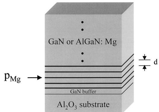
FIG. 1. Schematic diagram of Mg- $\delta$ -doped GaN or AlGaN, where  $d$  ( $=15 \text{ nm}$ ) and  $P_{\text{Mg}}$  denote, respectively, the distance between two  $\delta$ -planes and the two-dimensional Mg doping concentration.
